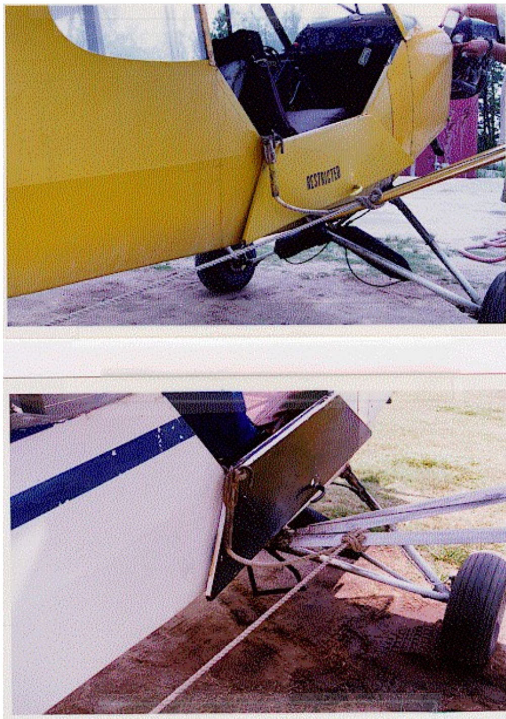
FIGURE 2-3. EXAMPLES OF A TYPICAL TOW ROPE CONFIGURATION, STOWED FOR DEPLOYMENT
