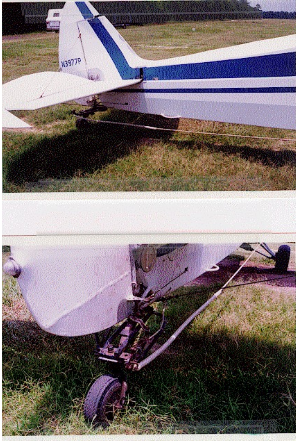
FIGURE 2-1. EXAMPLES OF A PLASTIC GARDEN HOSE INSTALLATION
