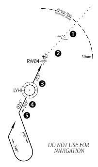
Figure 6-12 Sample Approach with Procedure Turn
