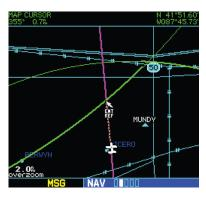
Figure 3-22 Using Pointer to Measure Distance and Bearing
