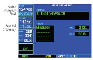
Figure 8-18 Frequency Moved to Active Field
