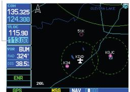
Figure 9-2 Tuning Cursor in VLOC Window
