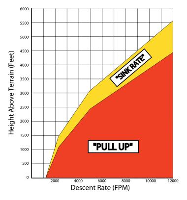
Figure 13-8 Excessive Descent Rate Alert Criteria
