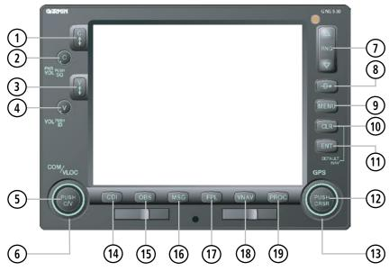
Figure 1-1 Keys and Knobs
