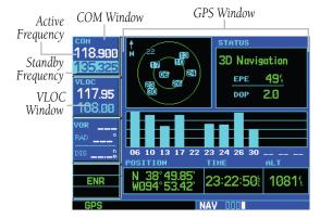
Figure 1-12 Standby Frequency 135.325 MHz
