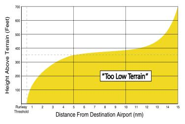
Figure 13-5 PDA Alerting Threshold
