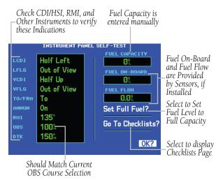
Figure 1-6 Instrument Panel Self-Test Page
