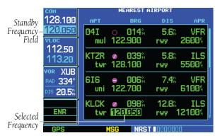
Figure 8-7 Frequency Moved to Standby Field
