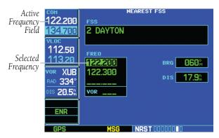
Figure 8-21 Frequency Moved to Active Field
