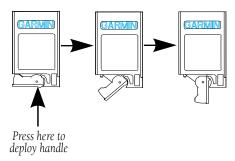
Figure A-3 Swing Arm Handle Operation
