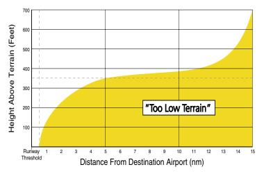
Figure 12-5 PDA Alerting Threshold
