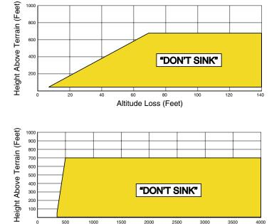
Figure 13-9 Negative Climb Rate (NCR) Alert Criteria
