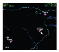
Figure 4-12 Panning Pointer Placed on Waypoint
