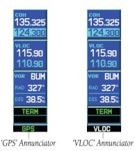
Figure 9-8 GPS and VLOC Annunciators
