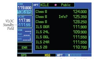
Figure 7-15 111.55 Moved to Standby Field
