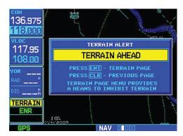
Figure 12-4 TERRAIN Caution Pop-up (Flashing)
