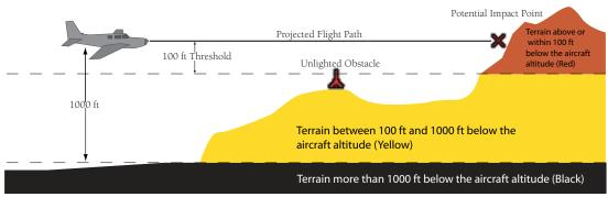
Figure 13-1 Terrain Altitude/Color Correlation for TAWS
