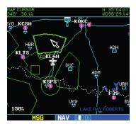
Figure 3-15 Select Airspace with Target Pointer
