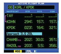
Figure 5-36 Procedure Header Highlighted
