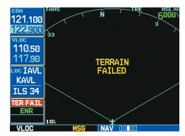
Figure 13-11: TAWS FAILED Display
