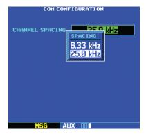
Figure 10-44 Channel Spacing Window
