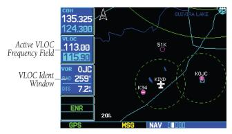
Figure 9-3 Frequency Moved to Active Field
