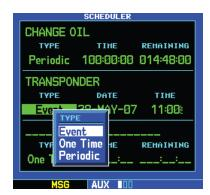
Figure 10-11 Type Field Highlighted
