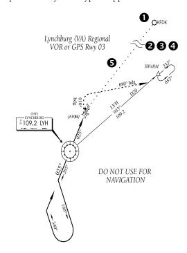
Figure 6-8 Sample Approach with Procedure Turn
