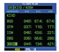
Figure 1-34 Enter Flight Plan Waypoints
