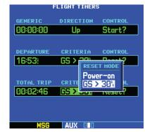
Figure 10-22 Total Trip Reset Mode Window
