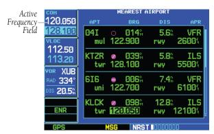
Figure 8-8 Frequency Moved to Active Field
