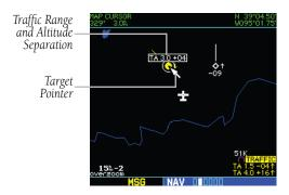
Figure 14-18 Traffic Range and Altitude Separation
