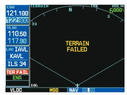
Figure 12-9: TERRAIN FAILED Display
