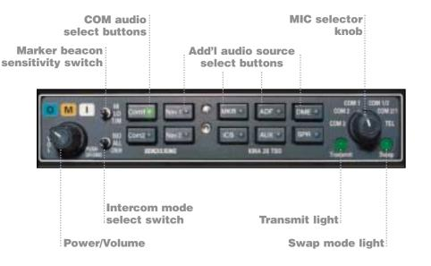
Then, there are such intercom features as IntelliVox®\* automatic squelch control, with separate voice activated squelch circuits for each microphone input to eliminate intercom squelch adjusting; the convenience of 6 intercom stations; and the real pleasure of stereo entertainment outputs.
